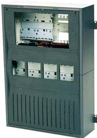
The CPH 0006 A can accommodate an MPC Operating and Display Unit with Panel Controller, up to six modules, two 12 V/45 Ah batteries, and a Power Supply. The Power Supply Bracket is fitted ex-works.
